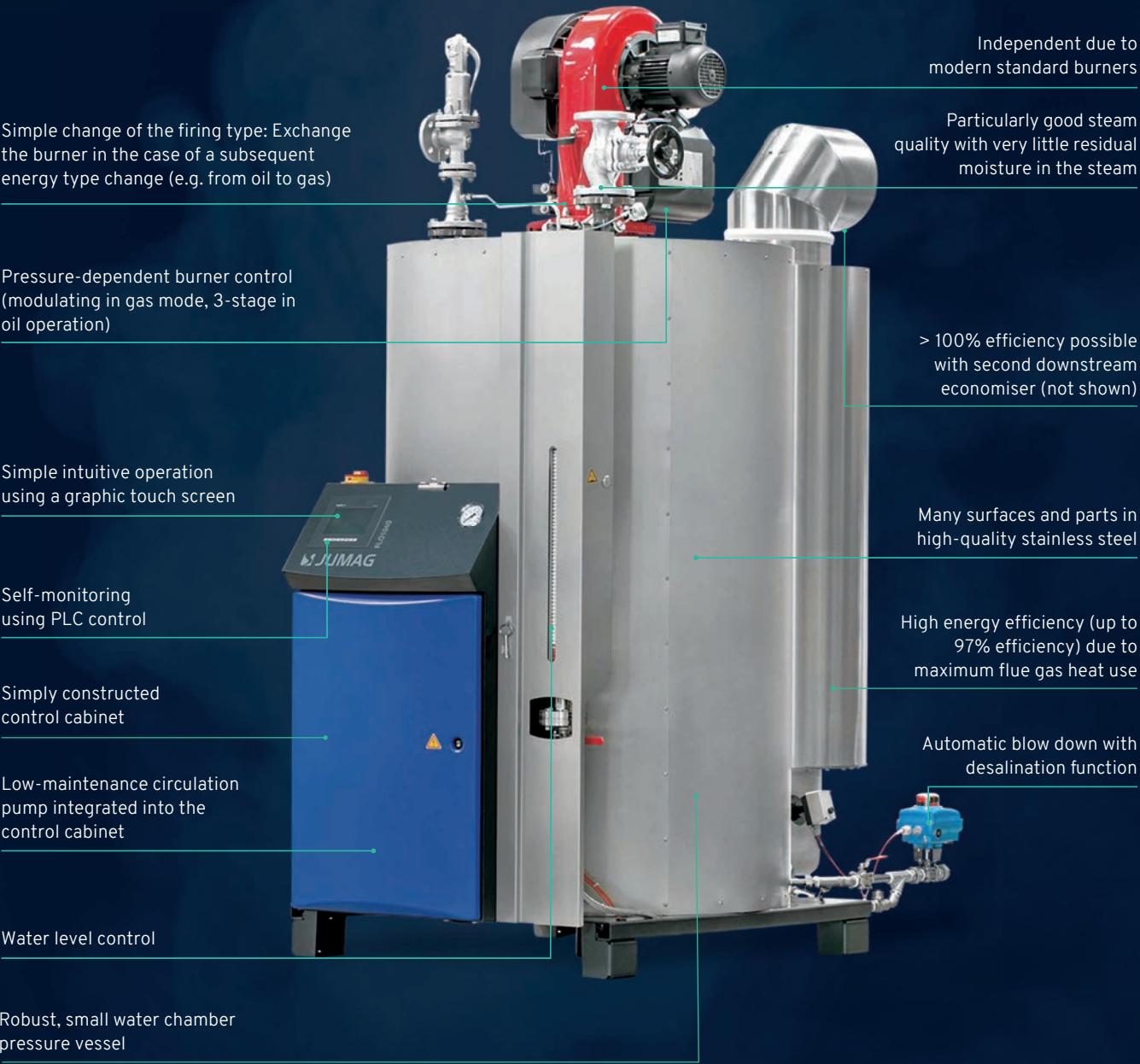
Fig.: JUMAG steam boiler FLO1060, example configuration
